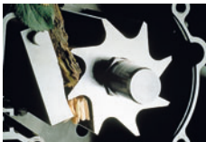
With the LH and ESK shredder, the cut material is drawn in by the rotating cutting wheel.
